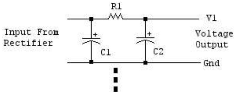
Resistors "R" may be substituted for chokes "L" wherever they appear, in any order and combination.
