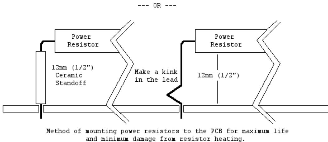
Please keep in mind also a respectable clearance between the PCB and chassis when mounting to avoid arcing from the pads or component leads to ground. Trimming the leads so there are no sharp points will also reduce the possibility of high voltage arcs and increase safety.
